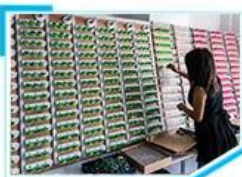
9. Aging test for travel charger
